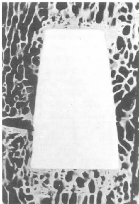
Fig. 3 Glass-ceramic A-W which substituted for a vertebra of a sheep and bonded to the surrounding cancellous bone. (contact radiomicrograph)
