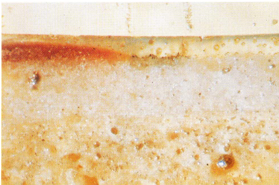
FIGURE 10 - Cross section of an Iznik tile illustrating a white slip coating over the underlying body together with areas of red and black pigment under the transparent lead alkali glaze.
