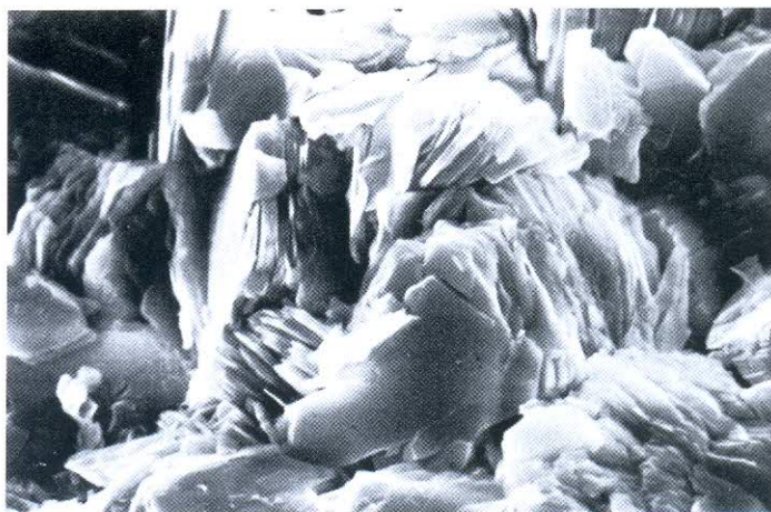
FIGURE 2 - The individual particles of kaolin are fine platelets with a thickness less than 0.5\ \mu\text{m} (3700X).
