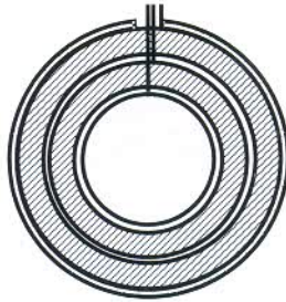
FIGURE 12 - A multilayer hollow spherical transducer prepared using a multiple coating process.
