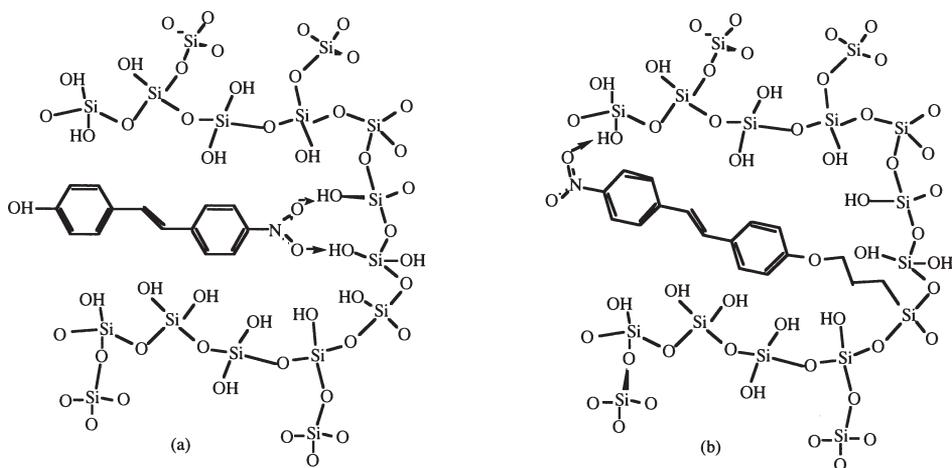
FIGURE 2 - Hybrid organic-silica nanocomposites for optics: the dye can weakly bind the surface of the silica matrix (a) or be covalently linked via functionalized alkoxydes (b).
